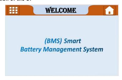
**Description:** Welcome page, power on for 3 seconds, used for program preparation communication and data exchange with BMS motherboard; Then enter the main status page;
